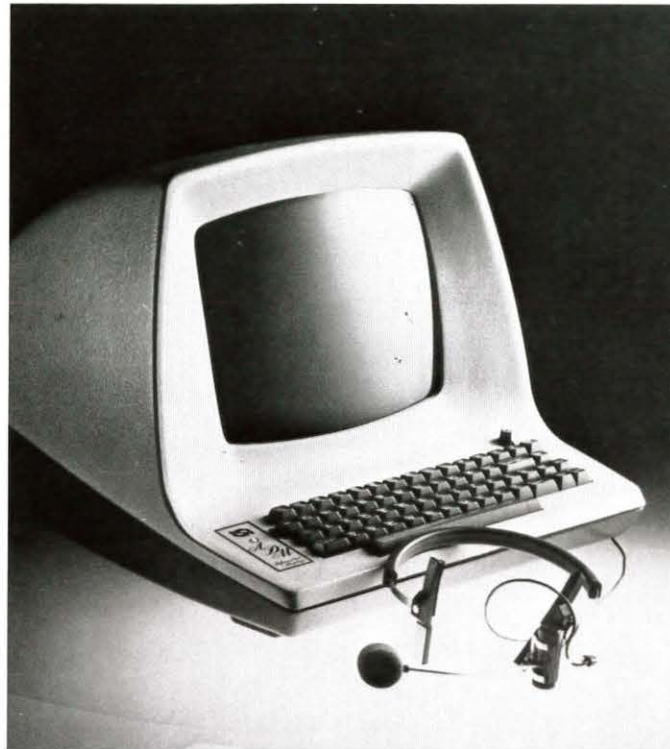
Lear Siegler's ADM 3A Dumb Terminal® video display is now capable of voice actuated data entry. This voice recognition unit was developed by Interstate Electronics, Inc. of Anaheim, California. The two companies recently signed a mutual development and marketing support agreement.
